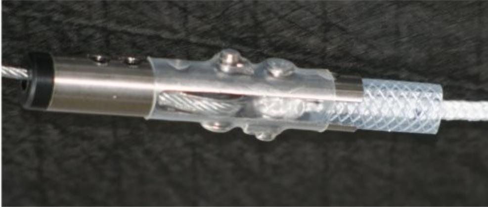
Felix writes: "The plastic tube has to be in the metal tube as well in order to protect the dyneema rope for sharp edges at the steel tube. It must be impossible to bring the dyneema rope in contact with the steel tube."
