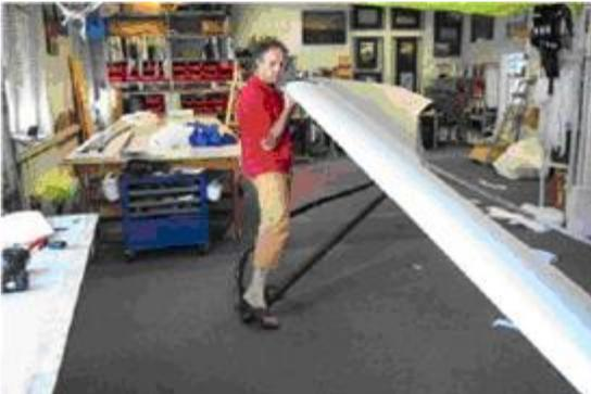
21.) Fix the nose cover. The Velcro has to be replaced if it loses strength. Don't fly with loose nose cover!
