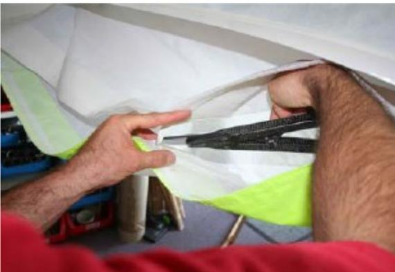
Before moving to the keel, ensure that the outer wing tube is inserted completely into the spar. Look through the hole in the sail.
