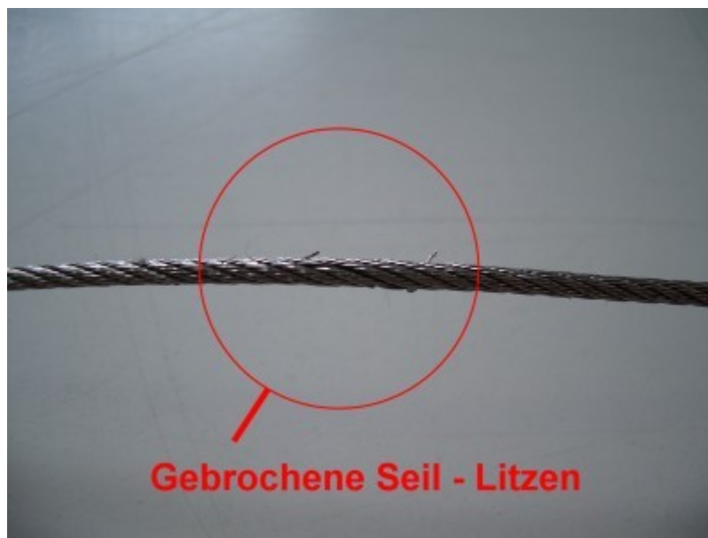
Picture 2 / damaged cable
